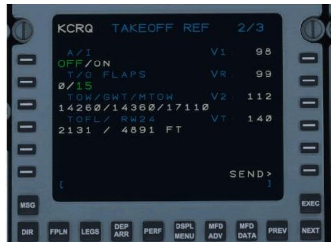
Once all performance data has been input, v-speeds should appear in the right-hand column. To get them to display on the PFD, press the **SEND** button. A message IN PROGRESS will appear followed by COMPLETE once the process has finished and they will appear in **MAGENTA** on the PFD below the speed tape.
