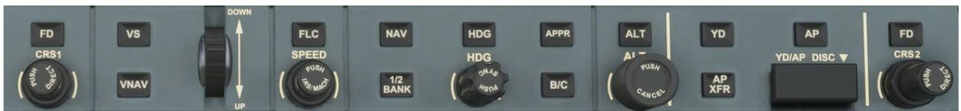
Fig 6.1 - Flight Guidance Panel
